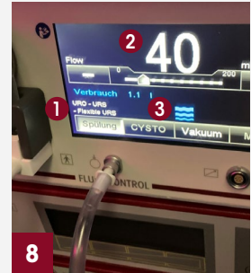
1) Pump ready for operation for Flexible URS 2) 40 ml/min is sufficient here 3) All three waves must be visible (for the best flow)
