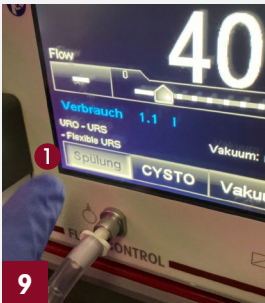
Starting with a cystoscope: If you are starting with a cystoscope, you need to switch to this mode briefly 1) First switch off the irrigation
