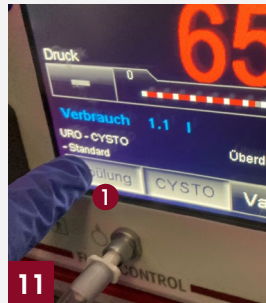
1) Activate irrigation The pump is now working in Cystoscopy mode
