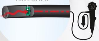
The CMOS Chip is positioned directly in the tip of the scope and transforms the analogue signal into a digital signal at the site of examination. This ensures noiseless and brilliant image transmission.
