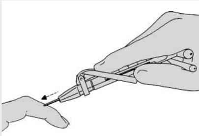
The wire is safely grasped with a gentle adduction of the thumb and is then screwed in or out with a simple rotational movement of the forearm.
