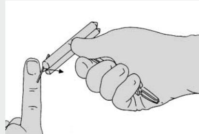
The handles feature bending devices for different wire diameters.
