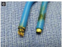
Figure. A: Photo shows two suction cautery tips after 30 seconds of cauterizing bovine renal tissue. The instrument on the bottom is coated with Electro Lube. B: Another photo shows two other tips after 30 seconds. The coated tip is on the right. C: Tips are seen after 60 seconds of cauterizing. The coated instrument is on the right.
