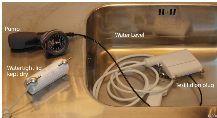
Figure 2. Example of a leakage testing setup with UA1414. Look for bubbles in the water.
