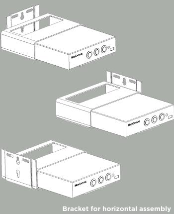
The additional bracket offers even more flexibility. Assemble your MVR® Recorder in any suitable position.
